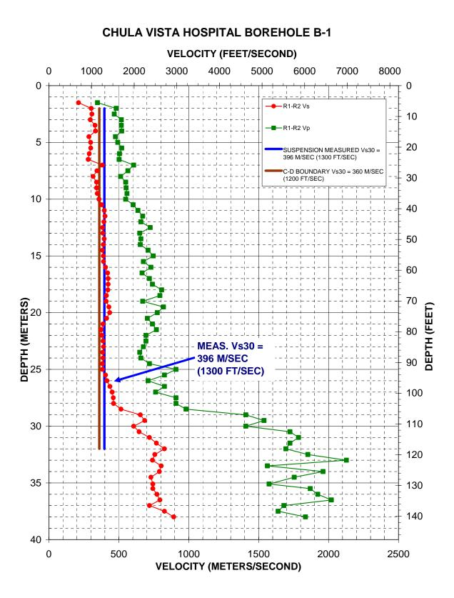
Figure 4: Boring B-1, Suspension R1-R2 P- and S<sub>H</sub>-wave velocities with Vs30 values
