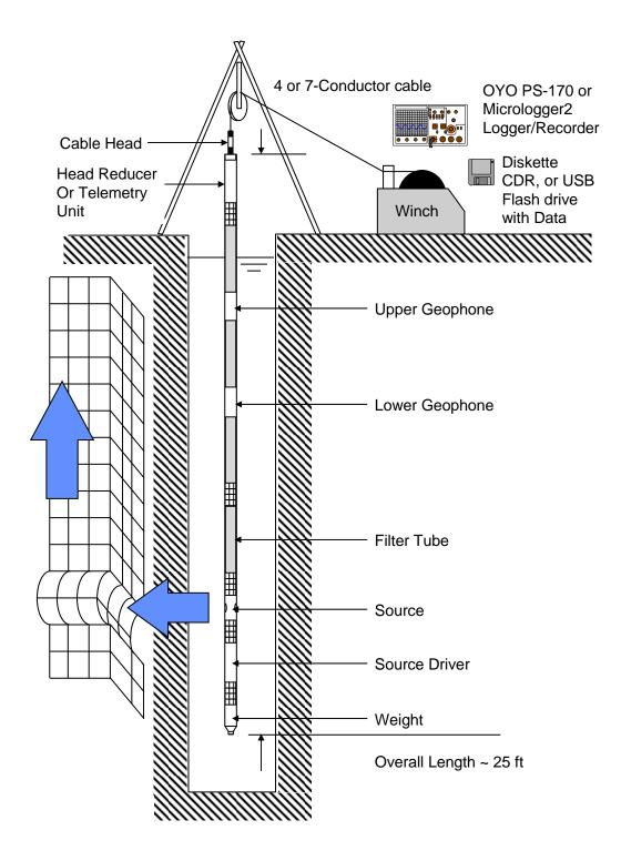
Figure 1: Concept illustration of P-S logging system
