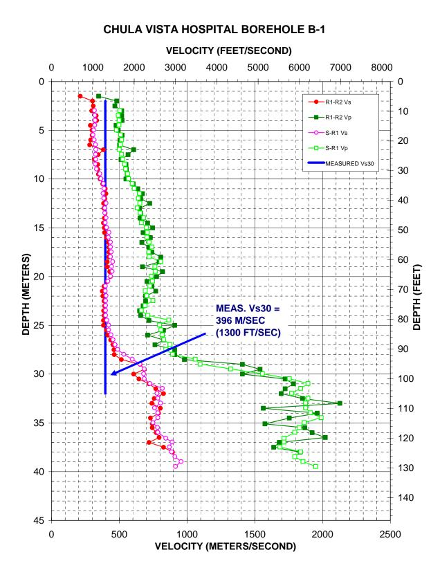
Figure A-1. Boring B-1, R1 - R2 high resolution analysis and S - R1 quality assurance analysis P- and  $S_H$ -wave data
